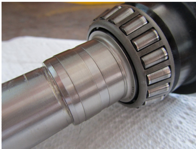
Repaired shaft with 2 SpeediSleeves,
